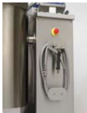
Hose reel mounted on the front of the pillar and hose connection on the top
